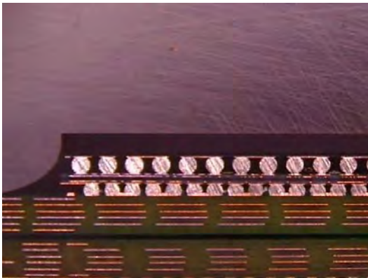
Figure 25. Cross section of Under-filled Module with forced rework on ENIG finish.
