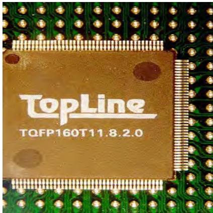
Figure 1. Illustrates the difference between QFP and BGA packages, showing an ultra fine- pitch 160 lead QFP (pitch 0.3 mm) on a background consisting of the bottom side of a 1.5 mm pitch PBGA with 225 interconnection solder balls. From this picture it is easy to understand the popularity this BGA package has received among the people in the assembly business. Note that there are five QFP leads for every BGA solder sphere.
