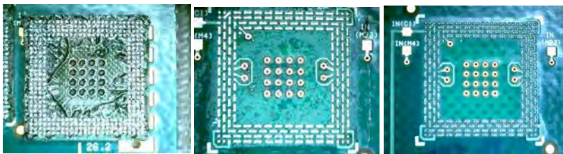
Figure 17. (Left) PoP rework site after removal of under-filled component. (Center) Site after complete under-fill removal. (Right) Site after complete under-fill removal and site redress.
